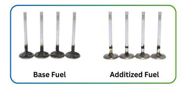
**GDI Fuel Injector Cleanliness:** NEW REQUIREMENT. This steady-state 120 hour engine dynamometer test evaluates the accumulation of deposits in injector nozzles, which can lead to poor fuel delivery, reduced fuel economy, and increased emissions. The test engine is a 2012-2013 GM LHU, a turbocharged four-cylinder inline engine with a 2.0-liter displacement.
