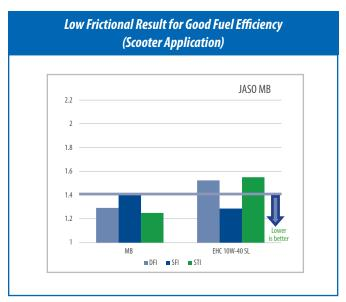
Robust JASO MA2 with base HiTEC® 22300 pack and can deliver JASO MB with HiTEC® 4716
